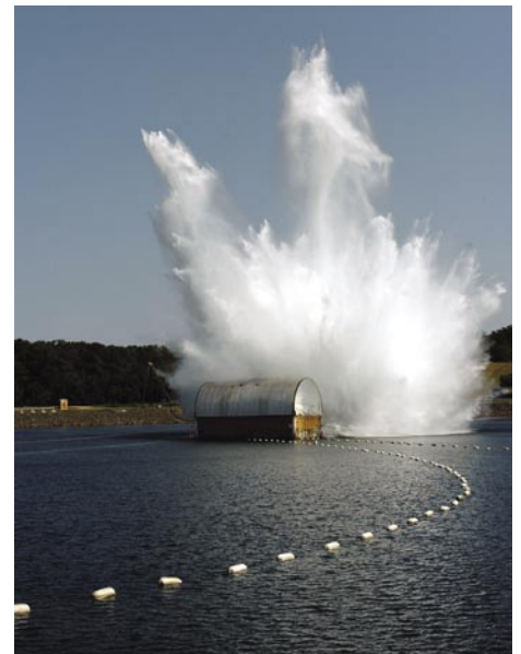
Shock qualification barge test of the VIRGINIA class Weapon Handling Module. (Photo courtesy of the Naval Undersea Warfare Center.)
